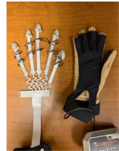
Figure 1. Flexi-Sensor Glove (Left) and CyberGlove (Right)
